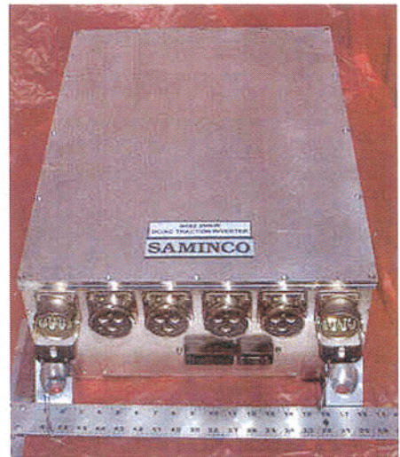
Figure K. 250 KW inverter oiled inverter for 3 phase Reuland AC induction motor
